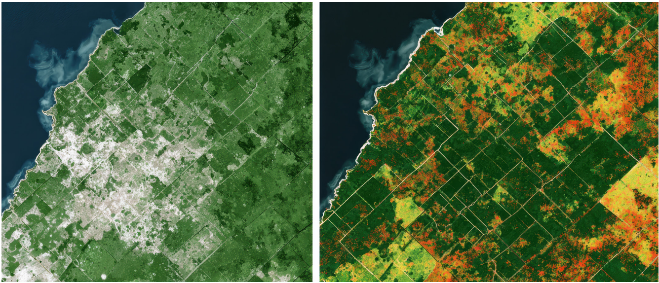
How NDVI helps map crop health based on reflectance of visible and near infra-red light
